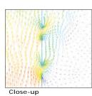
As seen in this CFD simulation, the air from the sonic vents tends to run along the surface of the duct and is not easy to control.
