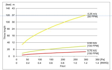
Throw data for a duct with nozzles shown at 0,75 m/s [150 fpm], 0,50 m/s [100 fpm] and 0,25 m/s [50 fpm] isothermal terminal velocity.
